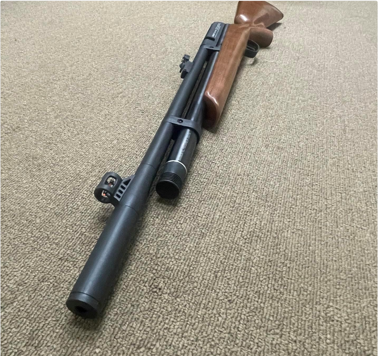
Image: Close-up view of the front section of the air rifle, showing the barrel and the air cylinder where the fill port is located.
