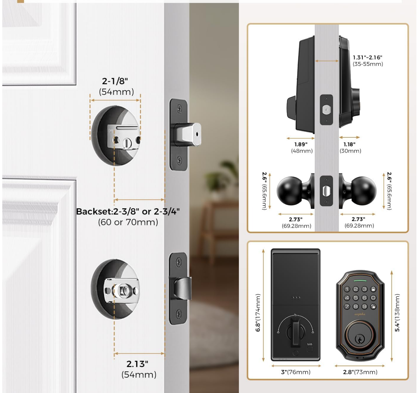
Image: A detailed diagram illustrating the dimensions and compatibility requirements for installing the ARPHA Keyless Entry Door Lock. It shows measurements for the bore hole ( 2\frac{1}{8}" or 54mm), backset ( 2\frac{3}{8}" or 60mm, or 2\frac{3}{4}" or 70mm), and the lock's overall size, ensuring proper fit on standard doors.
