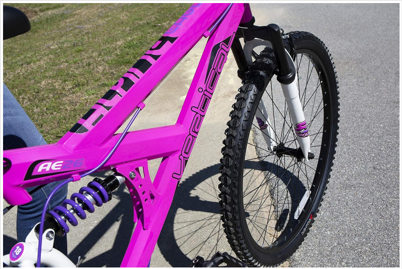
Image: Close-up of the bike frame, showing the AE26 model detail and the rear suspension system.
