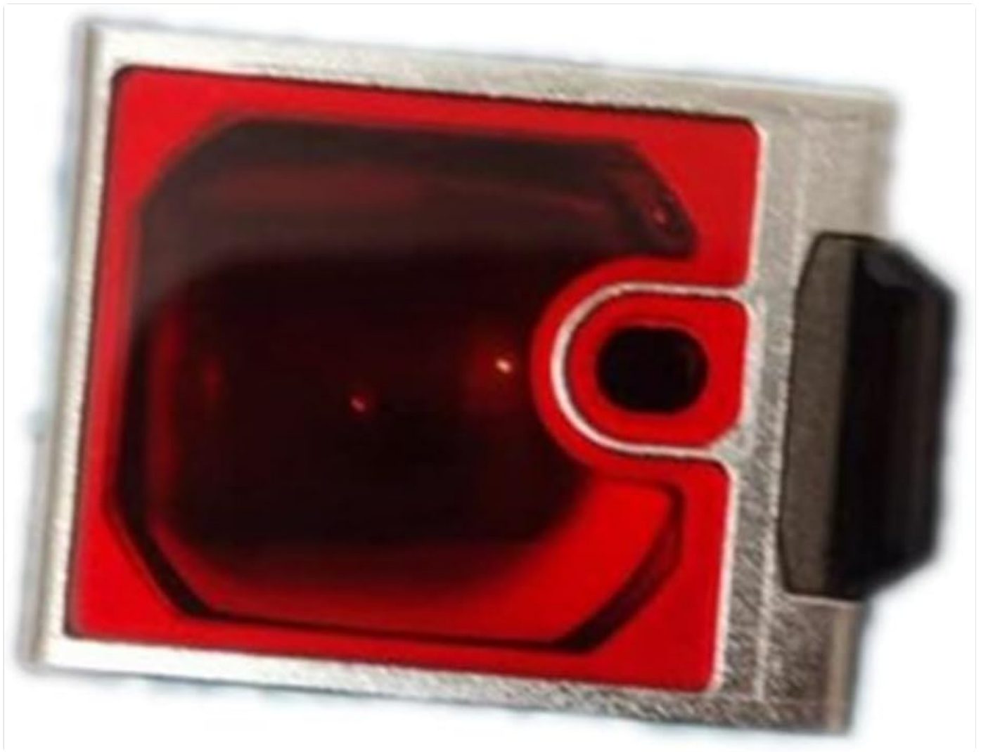
Figure 2: Side view of the LR-TB5000 Laser Sensor. This image highlights the red optical sensing element, which emits and receives the laser beam for displacement measurement and object detection. Proper alignment of this element is crucial for accurate operation.
