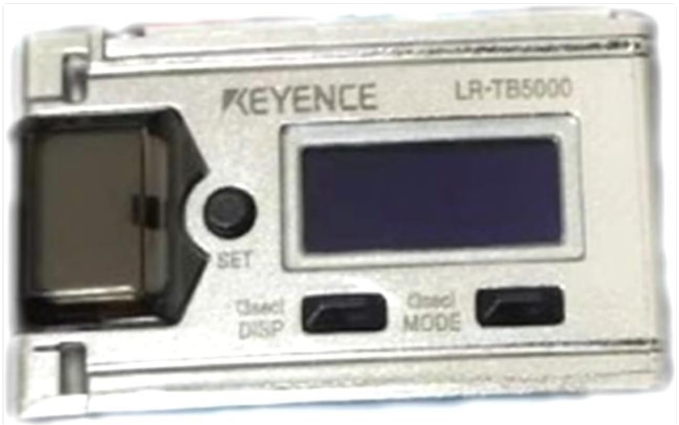
Figure 1: Front view of the LR-TB5000 Laser Sensor. This image shows the main body of the sensor, featuring a digital display screen and two control buttons labeled "SET" and "MODE/DISP". The sensor's compact design and integrated display allow for direct monitoring and configuration.
