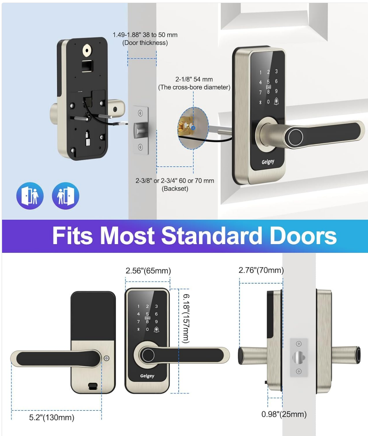
Figure 3: Door compatibility dimensions for the Gelgey F6 Smart Door Lock.
