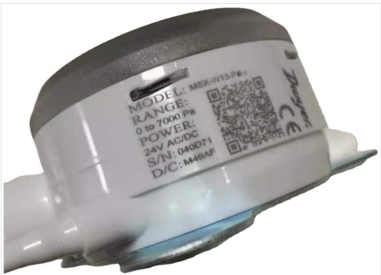
Figure 3.3: Side view of the sensor, featuring a label that specifies the model (MSX-W13-PA-LCD), pressure range (0 to 7000 Pa), and power requirements (24V AC/DC).
