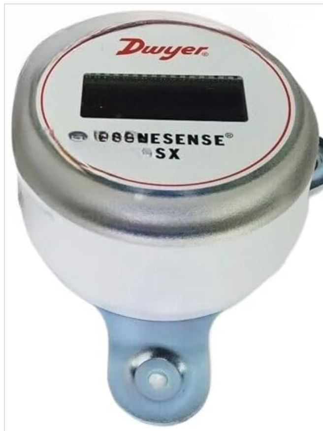
Figure 3.2: Detailed front view of the sensor, displaying the Dwyer logo and the LCD screen, which typically shows pressure readings.
