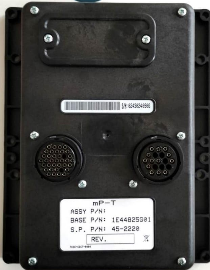
Figure 2: Rear view of the 45-2220 Microprocessor Controller. This view displays the two multi-pin electrical connectors and the product label with part numbers and serial number.
