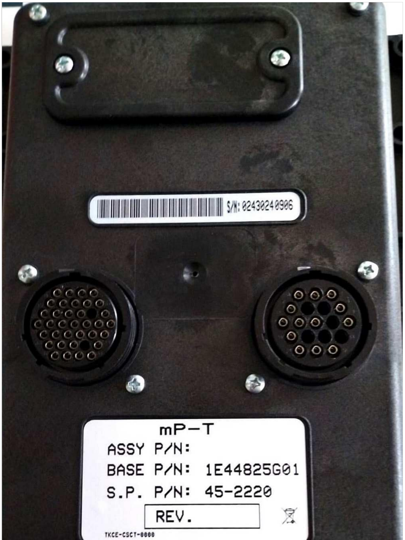
Figure 3: Close-up of the label and connectors on the rear of the 45-2220 Microprocessor Controller. The label clearly shows "mP-T", "ASSY P/N:", "BASE P/N: 1E44825G01", and "S.P. P/N: 45-2220", along with a barcode and serial number.
