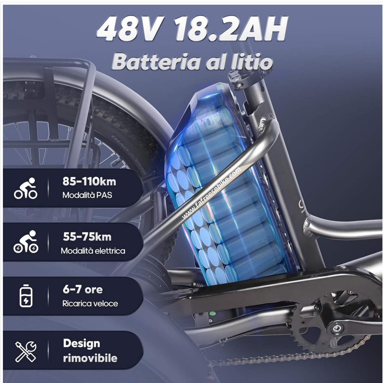
Image: Close-up of the 48V 18.2Ah lithium battery, highlighting its quick charge time and removable design.
