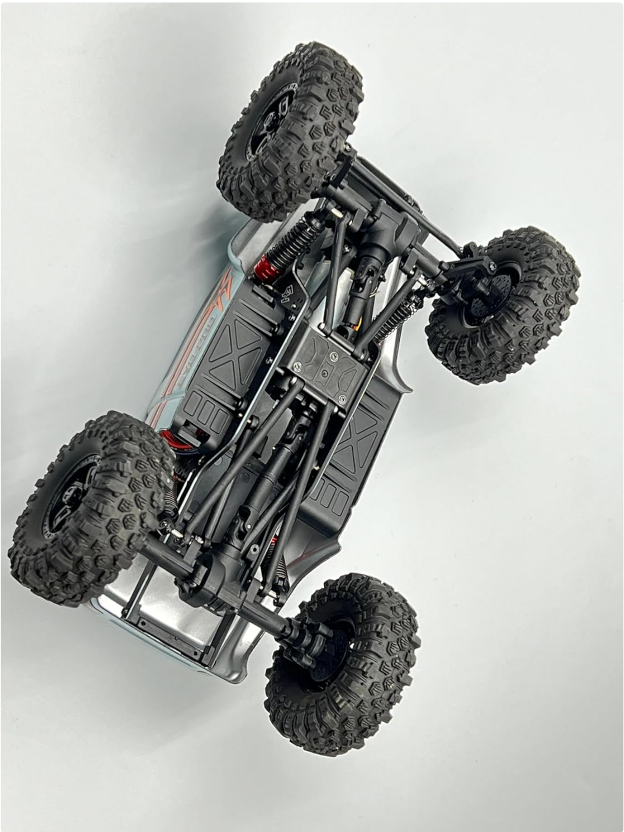
Image: Underside view of the CR-18P EVO PRO chassis, showing the drivetrain and suspension components.
