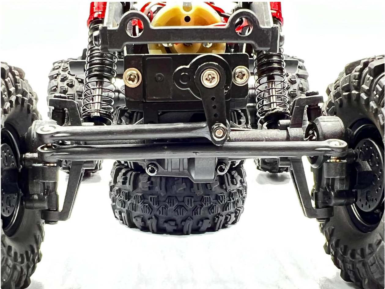
Image: Close-up of the front axle and the servo-on-axe (SOA) steering mechanism.
