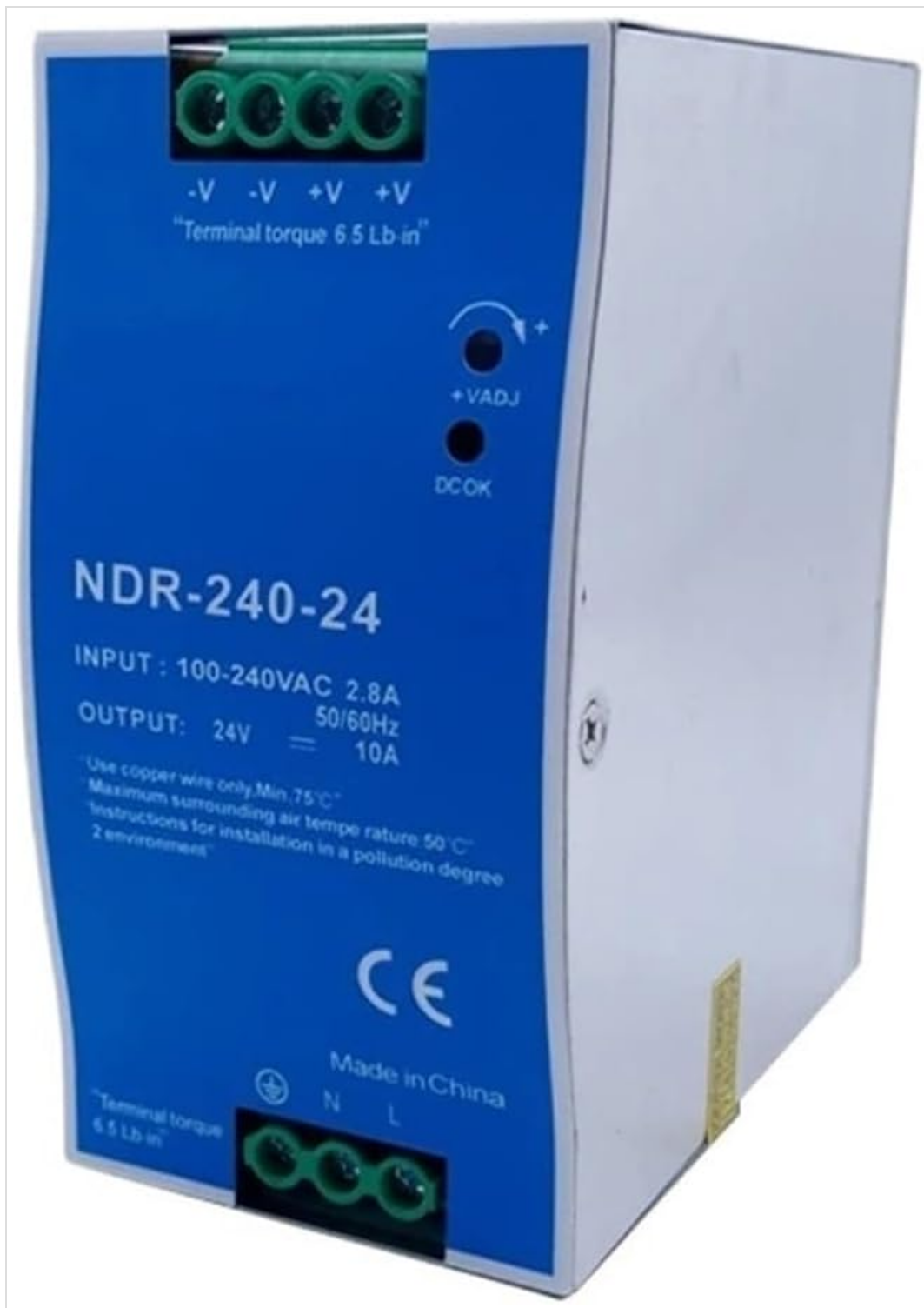
Figure 5.1: Close-up of the input and output terminal blocks, showing labels for AC input (N, L, Ground) and DC output (+V, -V).
