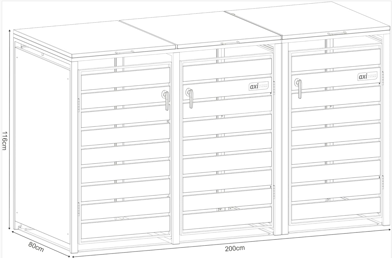
Image 6: Technical drawing illustrating the overall dimensions of the 3-container enclosure.
