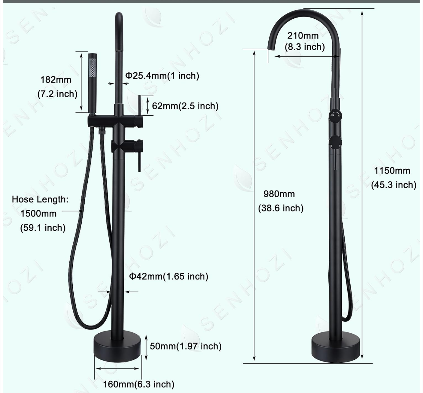
Image 7.1: Detailed dimensions of the Senhozi SE-3001-BK faucet, including height, spout reach, and hose length.
