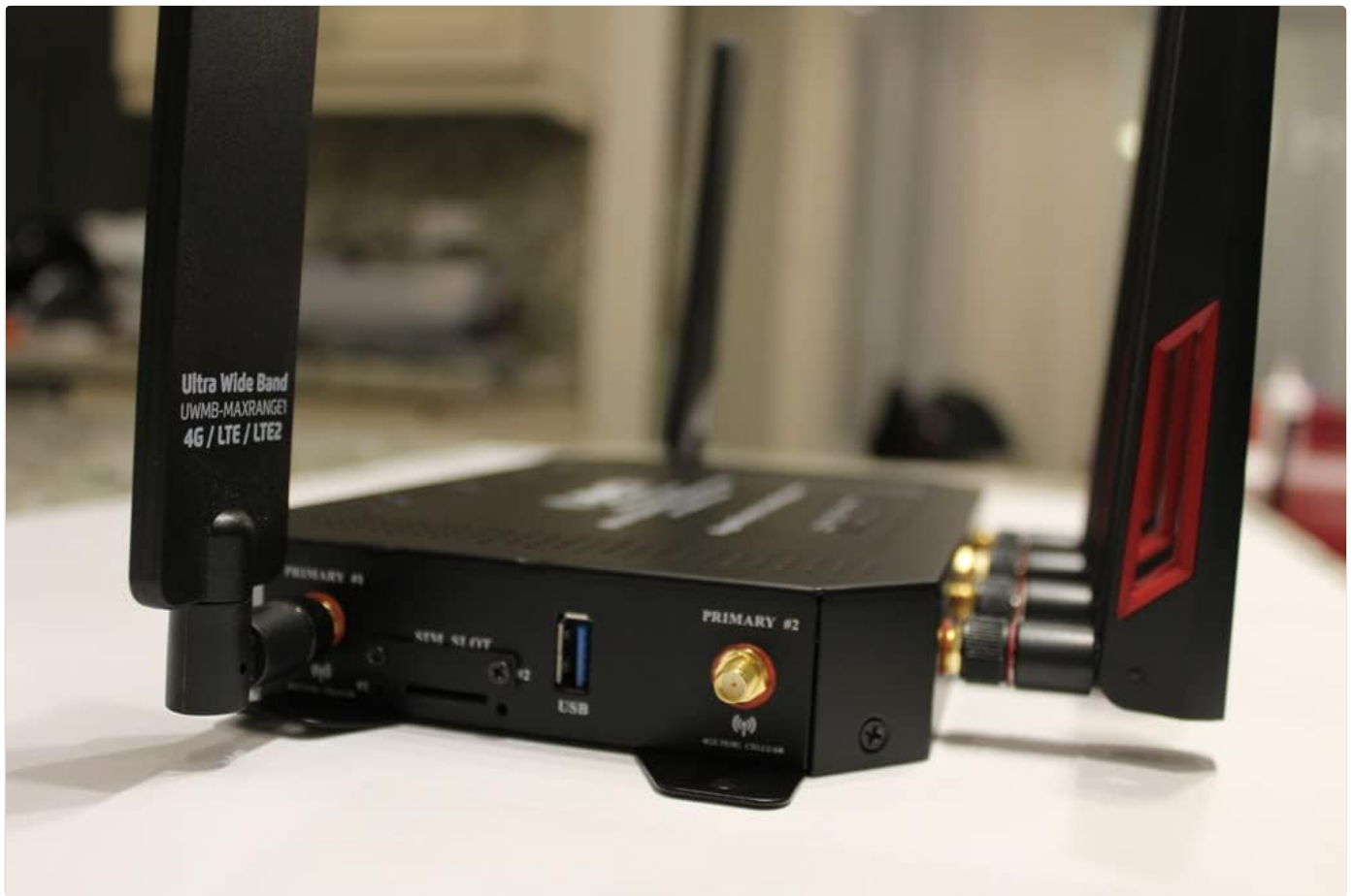
Figure 3: Side view of the MOFI5500-5GxLTE-RM520 router, illustrating the SIM card slot (SIM #1), USB port, SD card slot, and primary antenna connectors. This view is crucial for SIM card installation.
