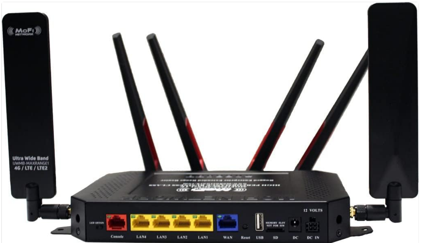
Figure 2: Rear panel of the MOFI5500-5GxLTE-RM520 router, highlighting the Console port, four Gigabit LAN ports, one Gigabit WAN port, Reset button, SD card slot, USB port, DC power input, and antenna connectors.
