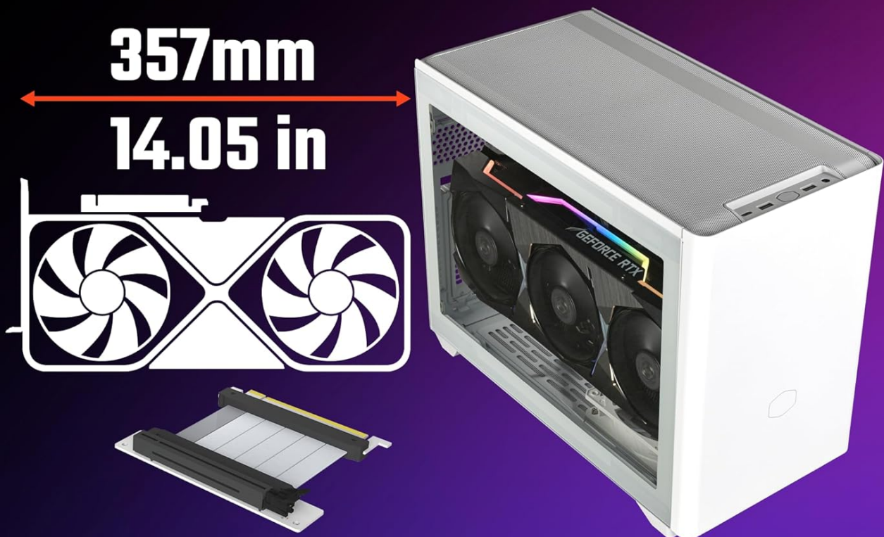
Image: A visual representation of a large graphics card (up to 357mm) mounted vertically within the Cooler Master NR200P V2 case, along with the included PCIe 4.0 riser cable.
