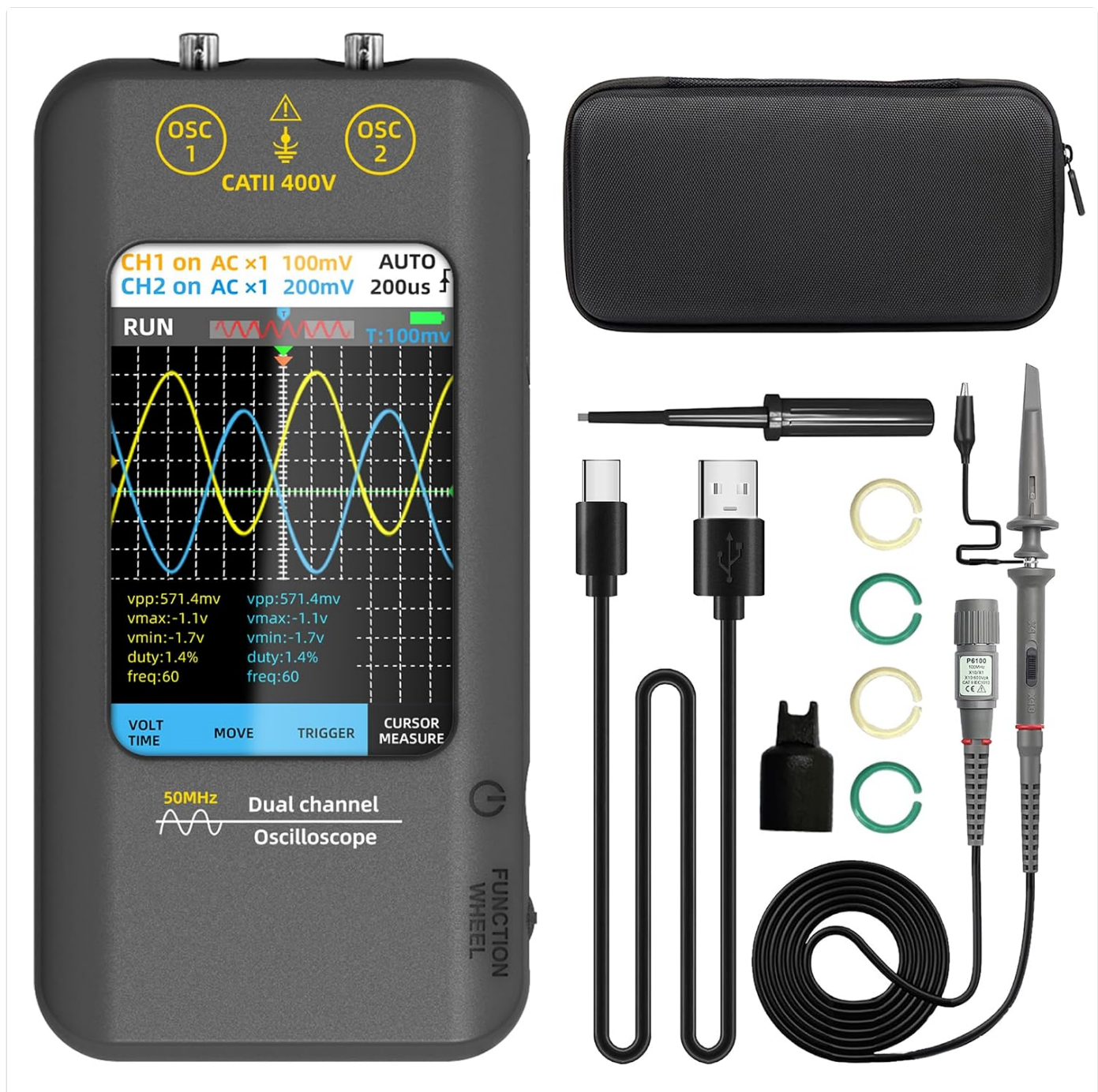
Figure 1.1: BSIDE O2 Dual Channel Handheld Oscilloscope and included accessories.
