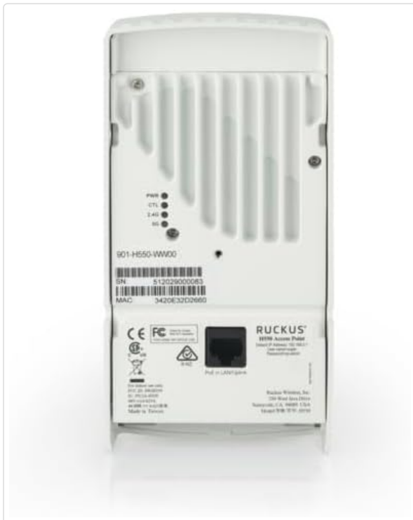
Figure 4: Rear view of the H550, displaying the product label with model number, serial number, MAC address, and regulatory compliance markings. Also visible are the mounting points and LED indicators for Power, Control, 2.4 GHz, and 5 GHz.
