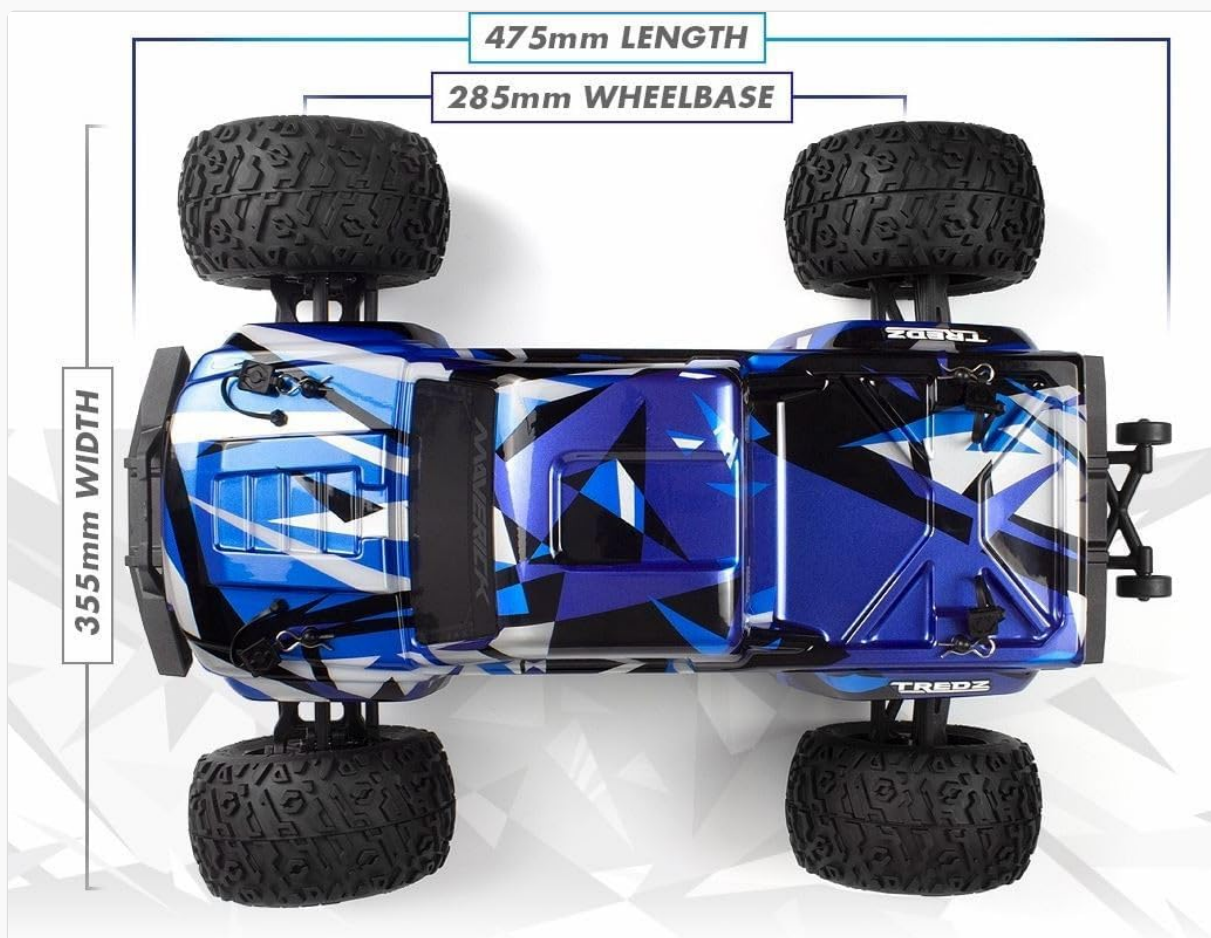
Diagram showing the length, width, and wheelbase dimensions of the Maverick Quantum2.
