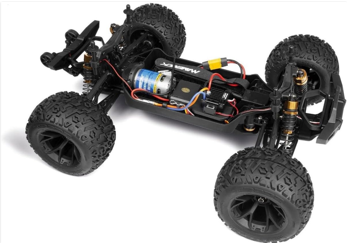
Internal view of the Maverick Quantum2 chassis, showing battery and electronics placement.
