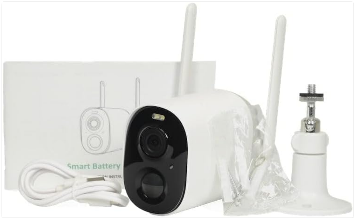
Figure 2.1: Package contents of the VICOHOME CG7 camera, showing the camera unit, mounting hardware, USB charging cable, and user manual.
