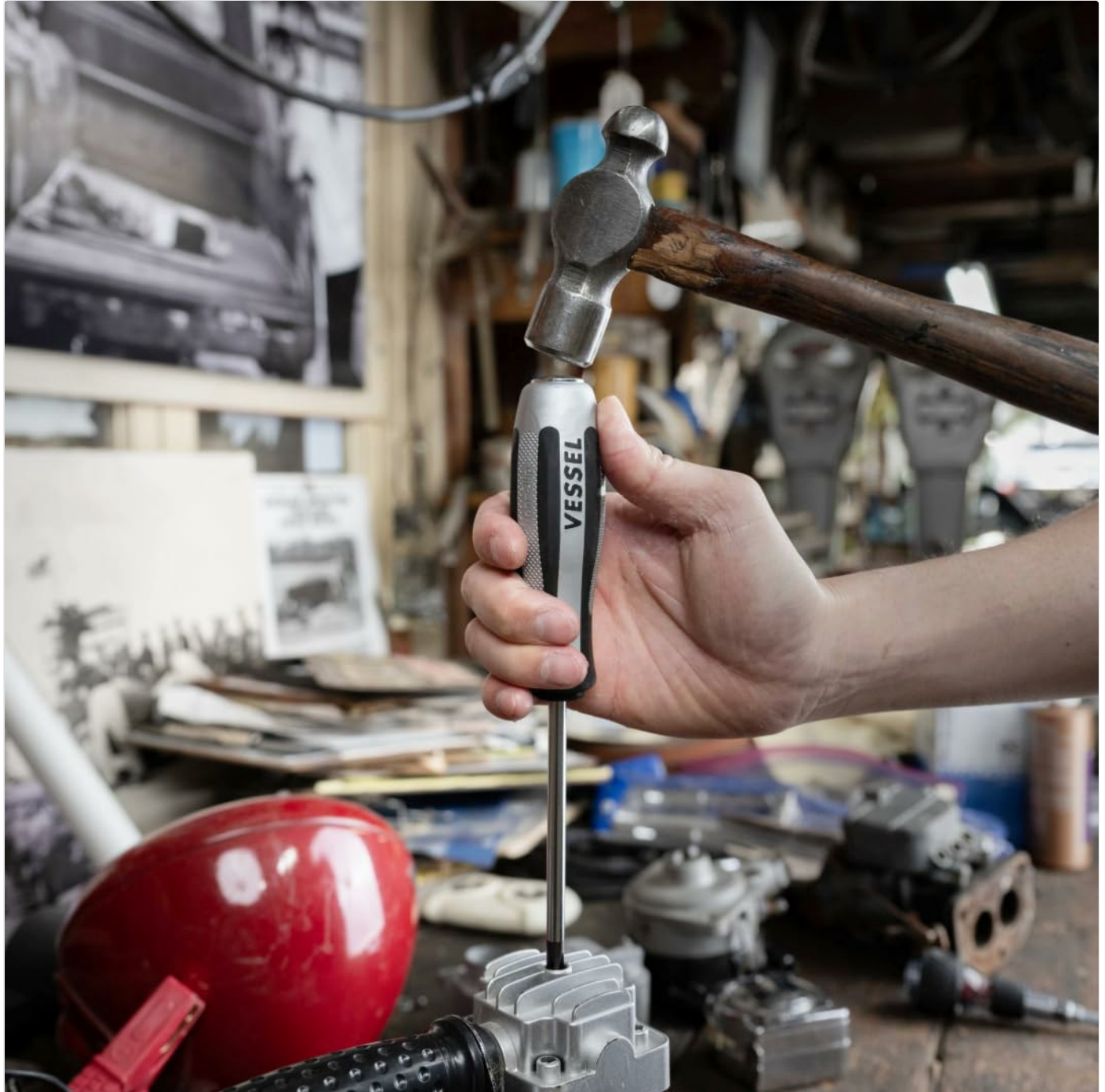
An image demonstrating the use of the silver-handled IMPACTA screwdriver, where a hammer is used to strike the steel cap, applying impact force to loosen a stubborn screw.
