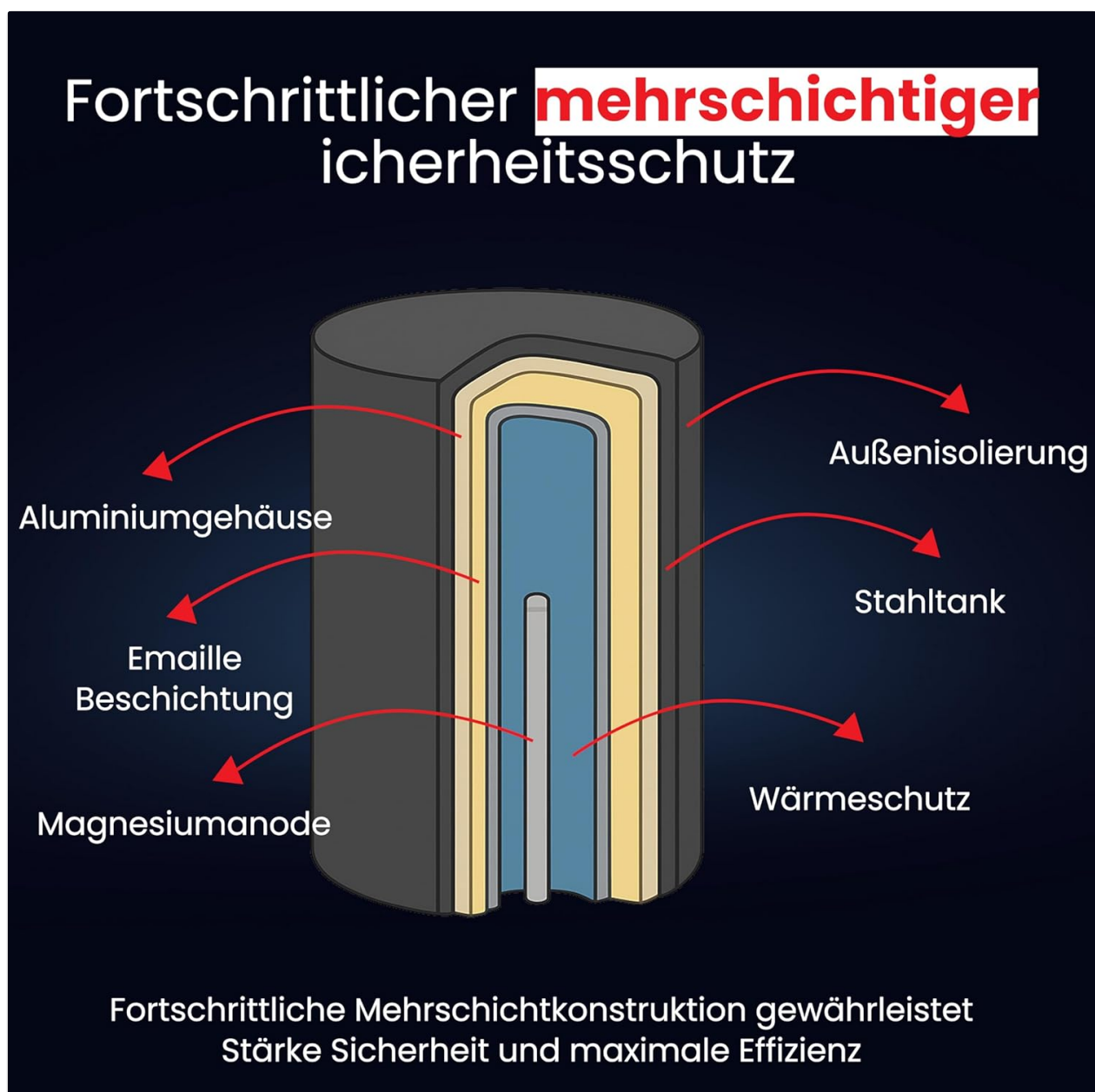
Figure 2: Cross-section diagram illustrating the multi-layered protective construction of the boiler, including the aluminum casing, enamel coating, magnesium anode, steel tank, external insulation, and thermal protection.
