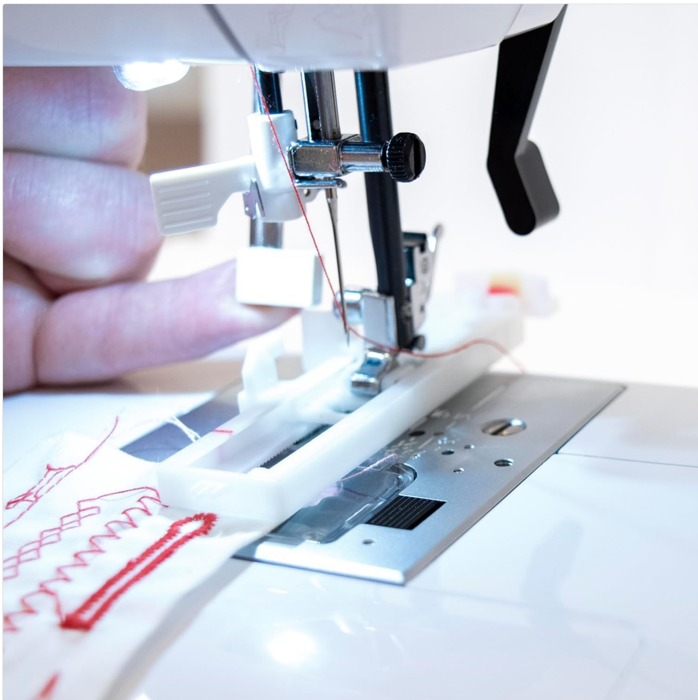
Figure 5.2: The automatic buttonhole foot in operation, demonstrating the machine's capability to create precise buttonholes.
