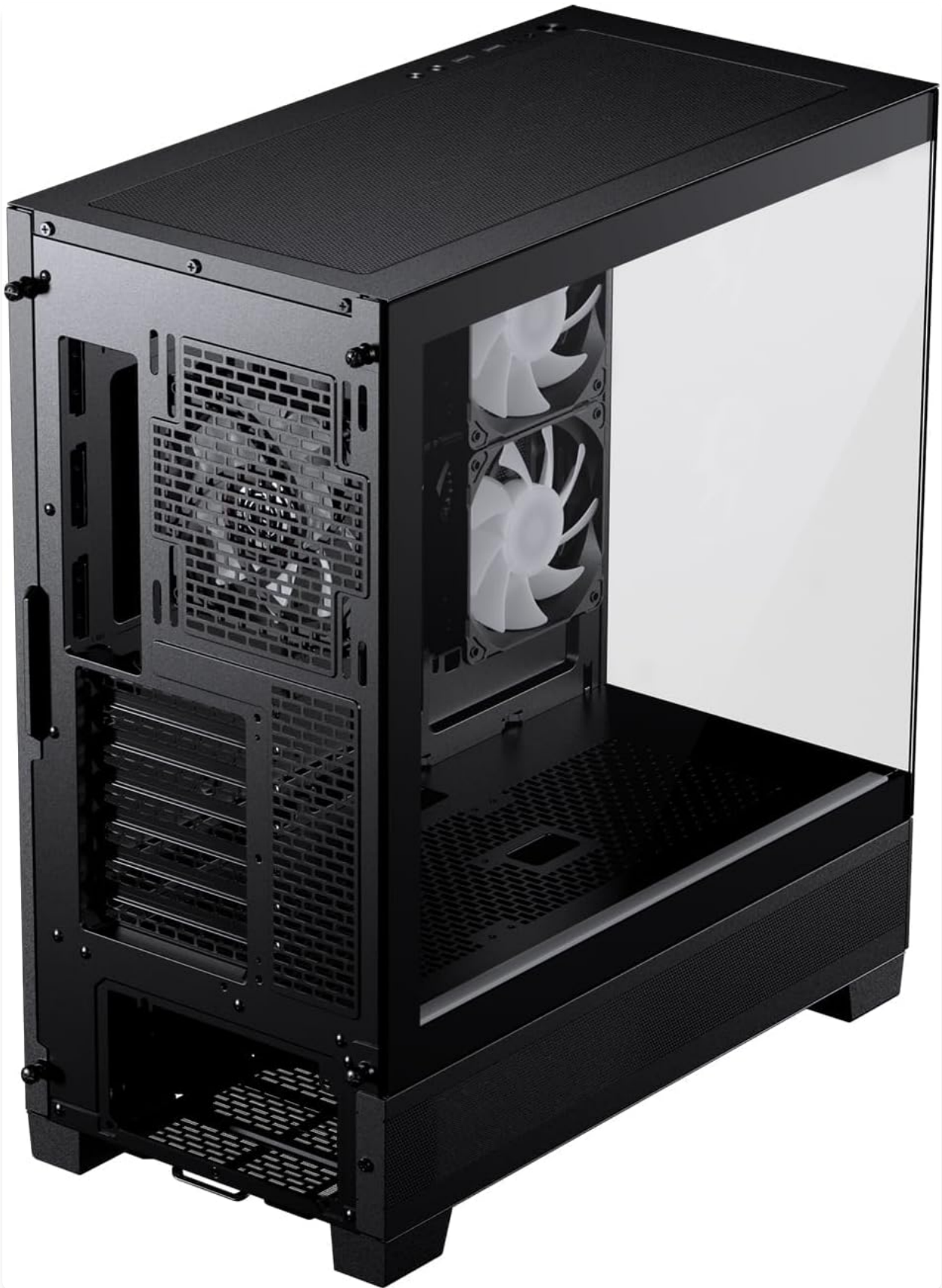
Image 3.3: Rear view illustrating cable management space.
