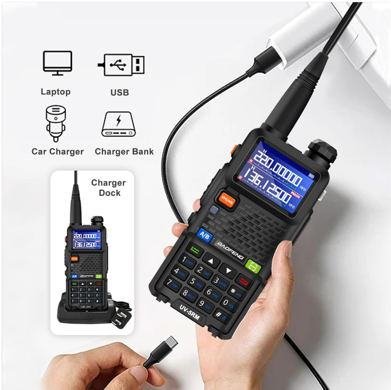
Image 3.1: The BAOFENG UV-5RM radio demonstrating both USB-C direct charging and charging using the desktop cradle.
