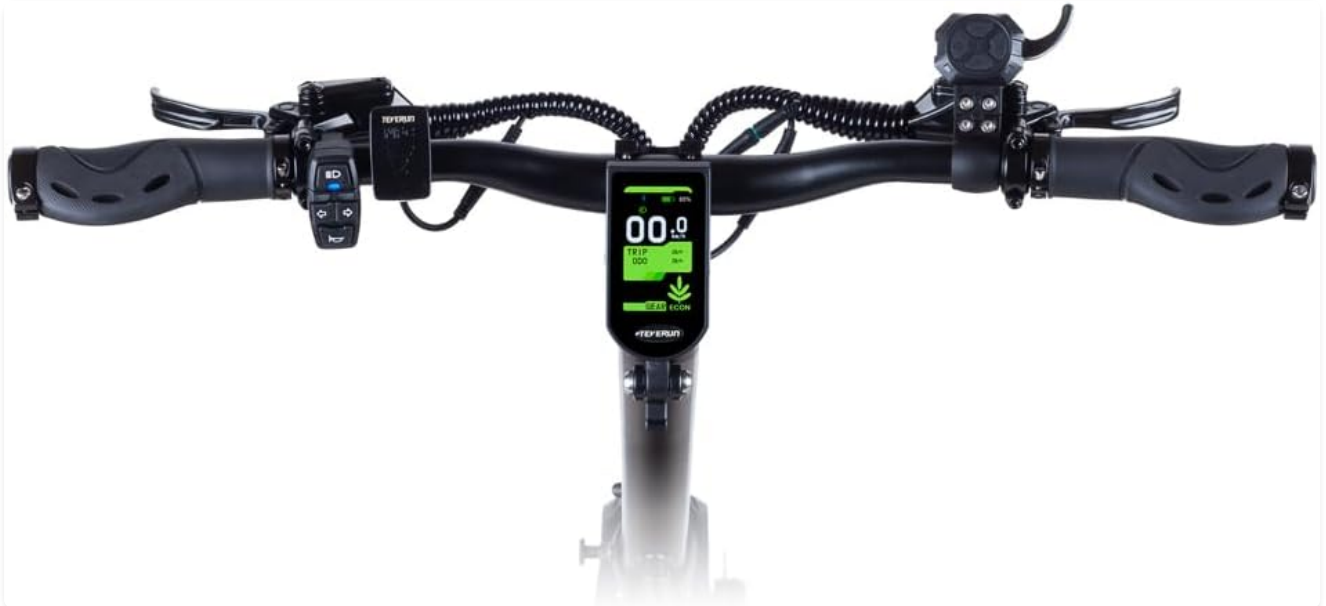
Figure 5.1: Top-down view of the handlebar assembly, showing the central display and control buttons.
