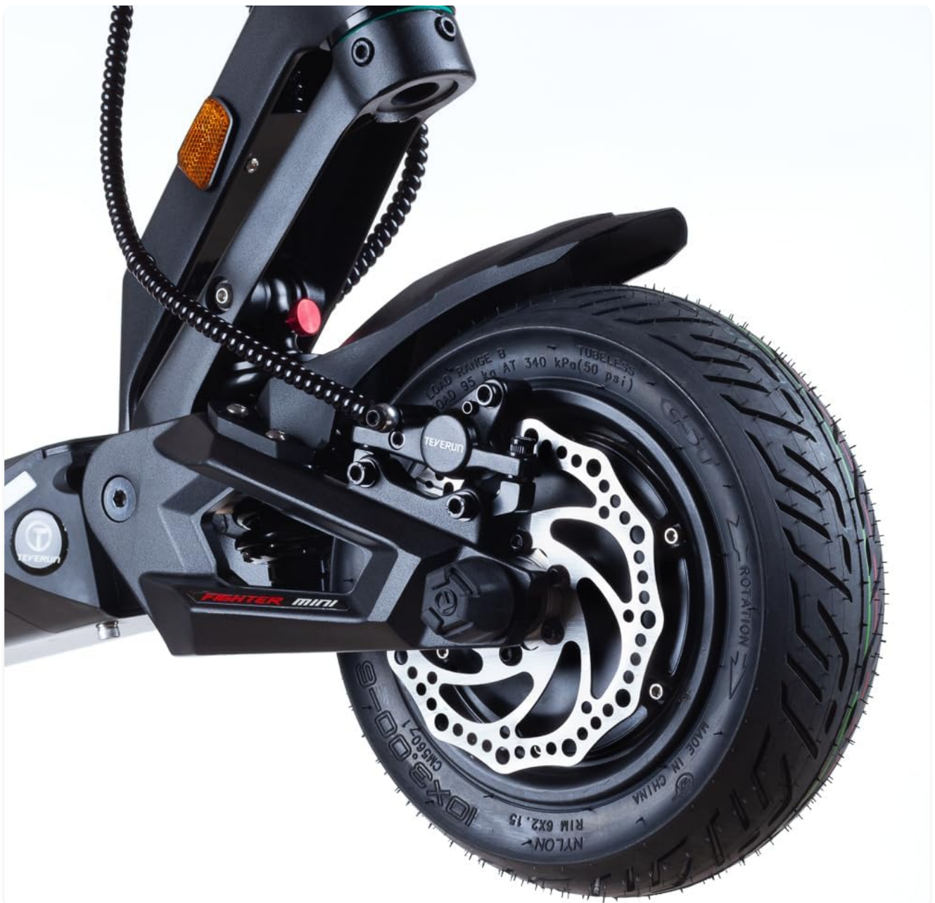
Figure 5.2: Close-up of the rear wheel, showcasing the robust hydraulic disc brake system.
