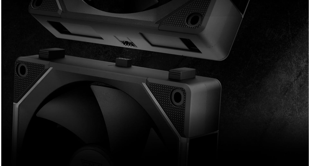
Image: Close-up of two GAMDIAS AEOLUS P2 fans demonstrating their interlocking mechanism for a cableless daisy chain connection.
