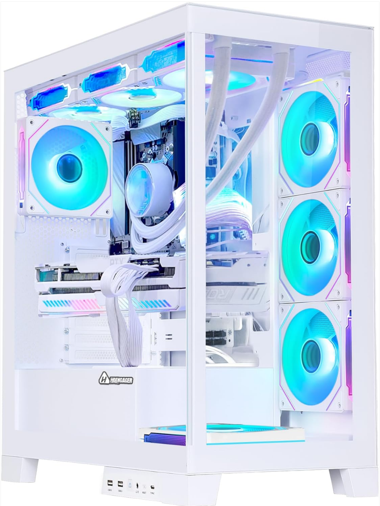
Image: Angled view of the HOENGAGER Superview Gaming PC, providing a clear look at the internal components, including the liquid cooler and case fans, which are crucial for maintaining optimal temperatures.
