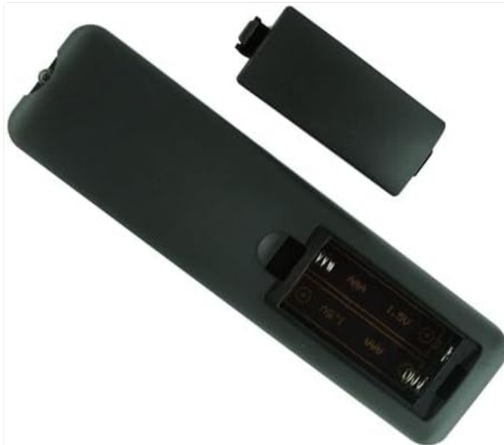
Figure 2: Back view of the remote control with the battery compartment open, illustrating battery insertion.
