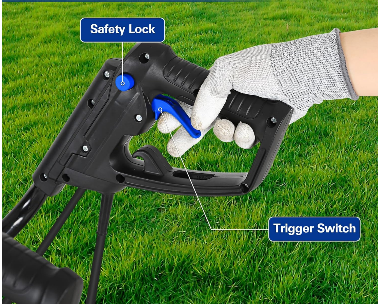
Figure 5.1: The safety lock button must be pressed before the trigger switch can be squeezed to operate the tiller.
