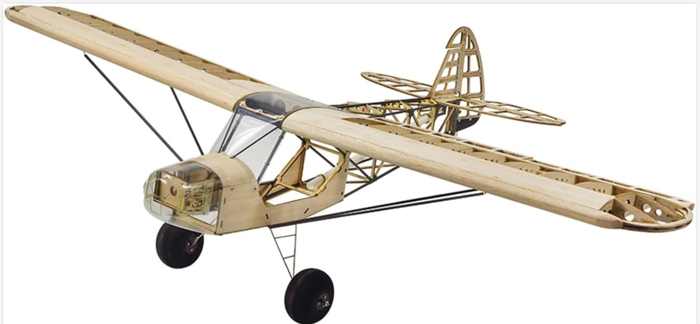
Image: The fully assembled S38 Savage Bobber balsa wood RC airplane, showcasing its classic design and wooden frame.
