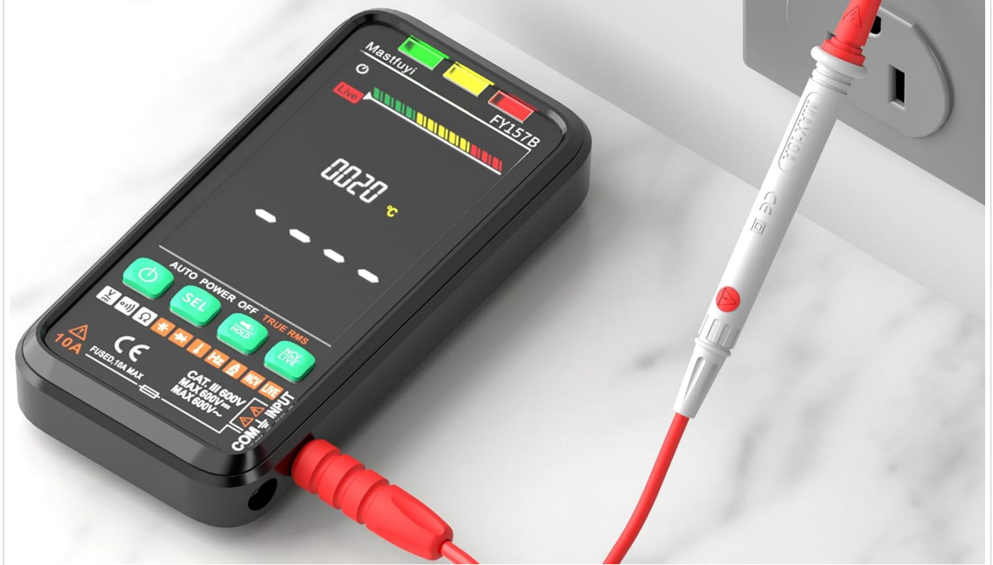
Figure 5.4: Using LIVE mode to identify the hot wire in an electrical socket.
