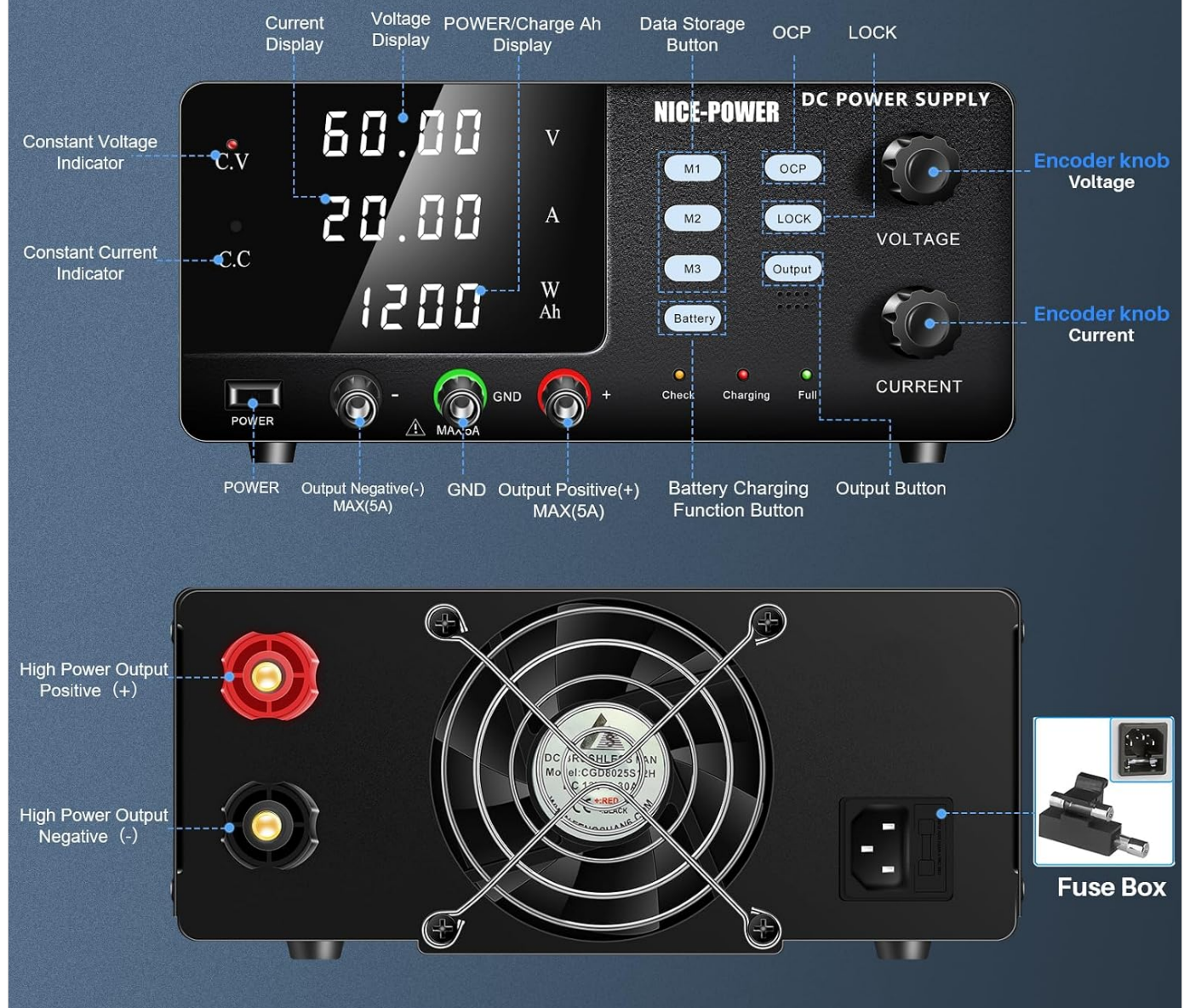
Figure 1: Front and Rear Panel Overview. This image displays the front panel with digital readouts for voltage, current, power, and Ah, along with control knobs for voltage and current, memory buttons (M1, M2, M3), OCP, Lock, Output, and Battery functions. The rear panel shows the cooling fan, AC power input, high power output terminals, and fuse box.
