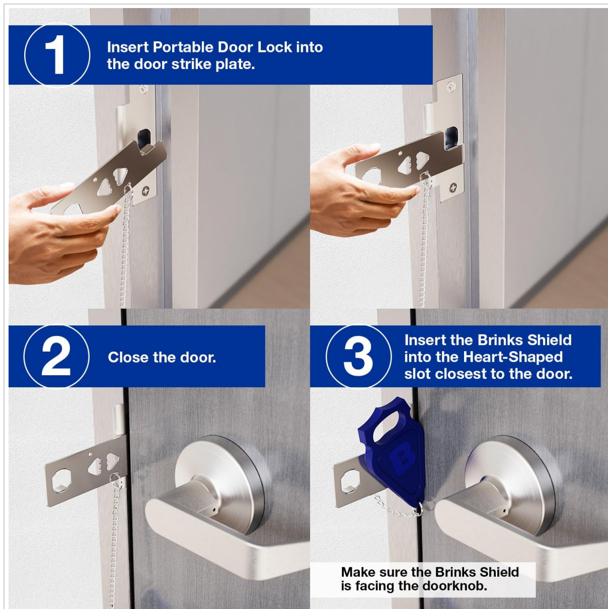
Figure 4.1: Visual guide for installing the BRINKS Portable Security Door Lock. Steps include inserting the metal piece into the strike plate, closing the door, and securing the blue shield.
