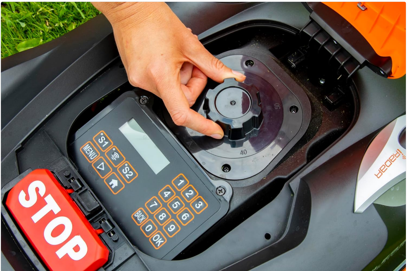
Image: Cutting Height Adjustment. A hand is shown turning a dial on the top of the robotic mower, which is used to adjust the cutting height of the blades. The dial has numerical markings, indicating different height settings.
