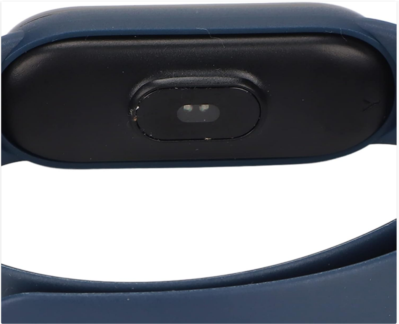
Image: A close-up view of the back of the smart bracelet, highlighting the optical sensor used for heart rate monitoring.
