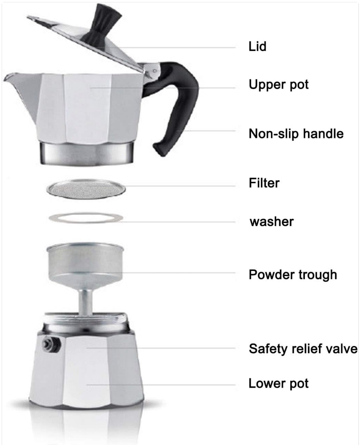
Image: An exploded diagram illustrating the individual components of the moka pot.
