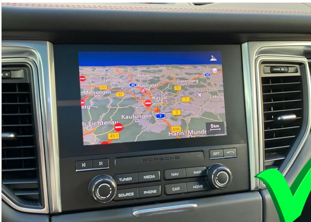
Figure 3.1: Visual guide for identifying PCM 3.1 (incompatible, marked with a red X) versus PCM 4.0 (compatible, marked with a green checkmark) in a Porsche Macan dashboard.
