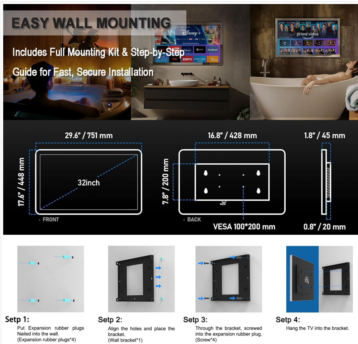
Figure 5.1: Easy Wall Mounting Guide. This diagram illustrates the dimensions of the 32-inch mirror TV and its wall bracket, along with four steps for secure installation using expansion plugs and screws.
