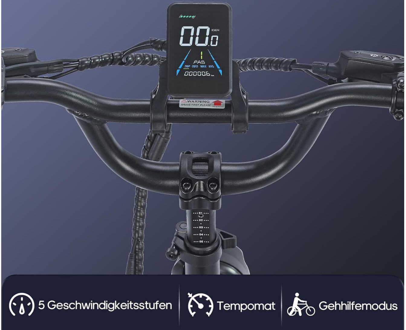
Image: The Fafrees F20 Mate's LCD color display, showing speed, battery, and pedal assist levels, along with controls for various functions.
