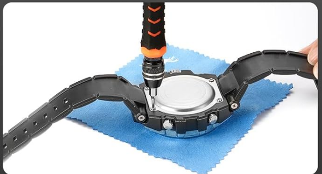
Figure 8: Demonstrations for opening different watch back types using the appropriate tools.
