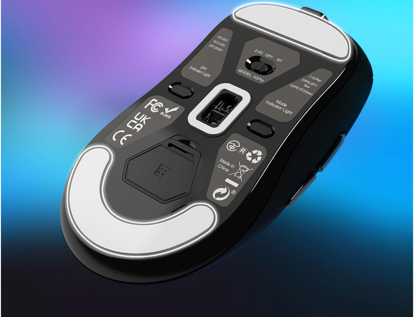
Figure 5: The X3PRO features 100% virgin grade PTFE feet for smooth gliding.
