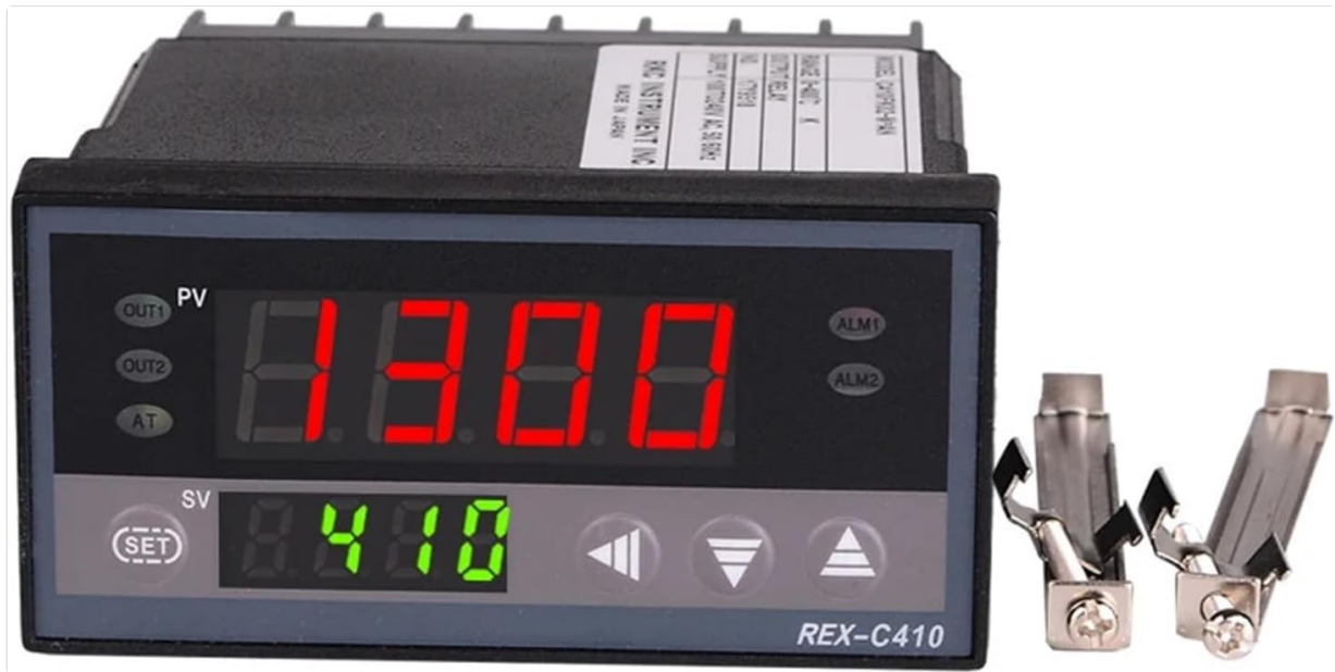
Figure 4.1: The REX-C410 controller shown with its included mounting clips, which secure the unit into a panel cutout.
