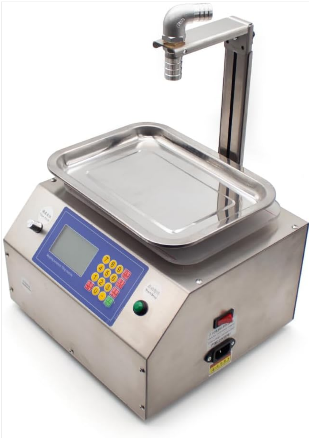
Figure 4.2: Close-up of the control panel and stainless steel weighing platform. The control panel features a digital display and a numeric keypad for setting parameters.
