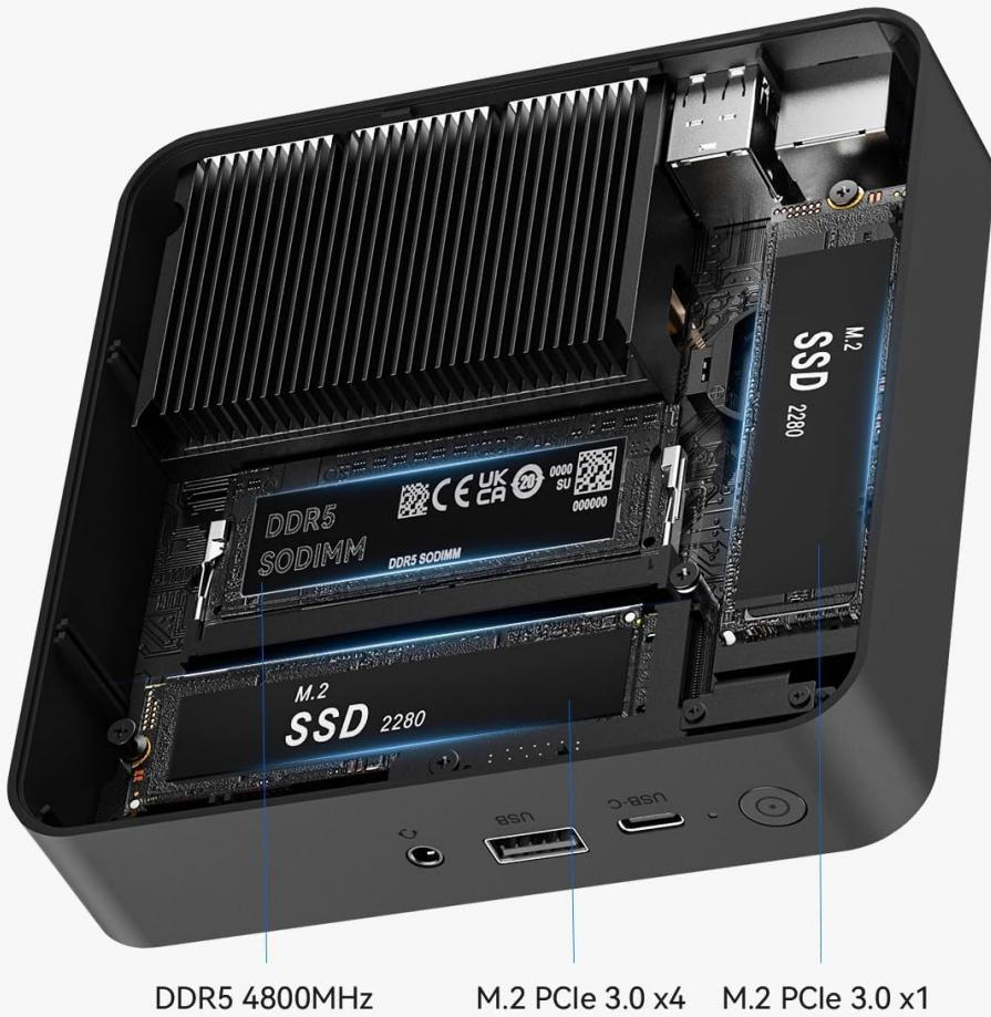
This image provides an internal view of the mini PC, highlighting the DDR5 SODIMM memory module and the two M.2 SSD slots, one M.2 PCIe 3.0 x4 and one M.2 PCIe 3.0 x1.
