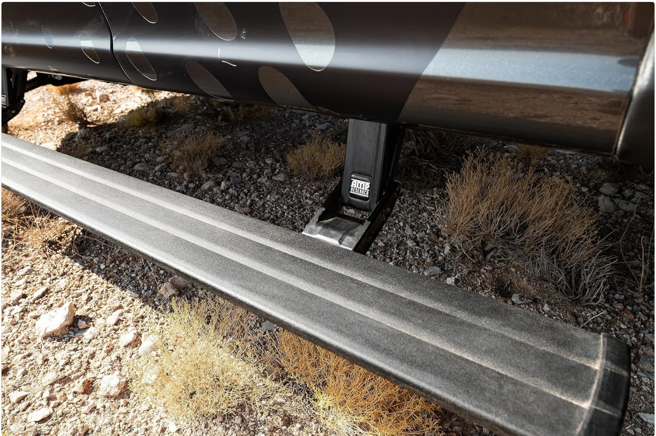
Image 5: Inspect the linkage mechanism for smooth operation and proper lubrication.
