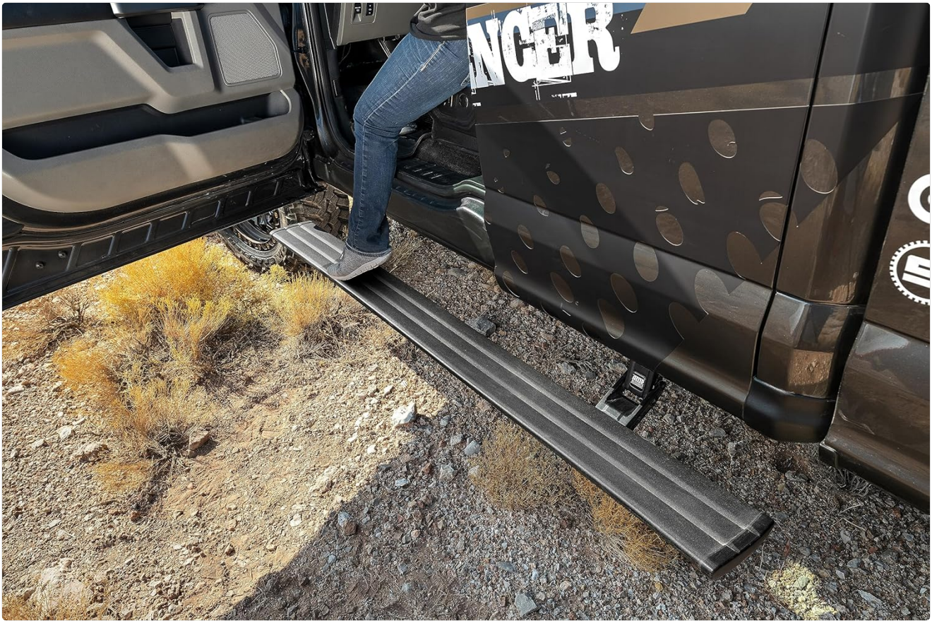
Image 2: The PowerStep extends to provide a convenient step for vehicle entry.
