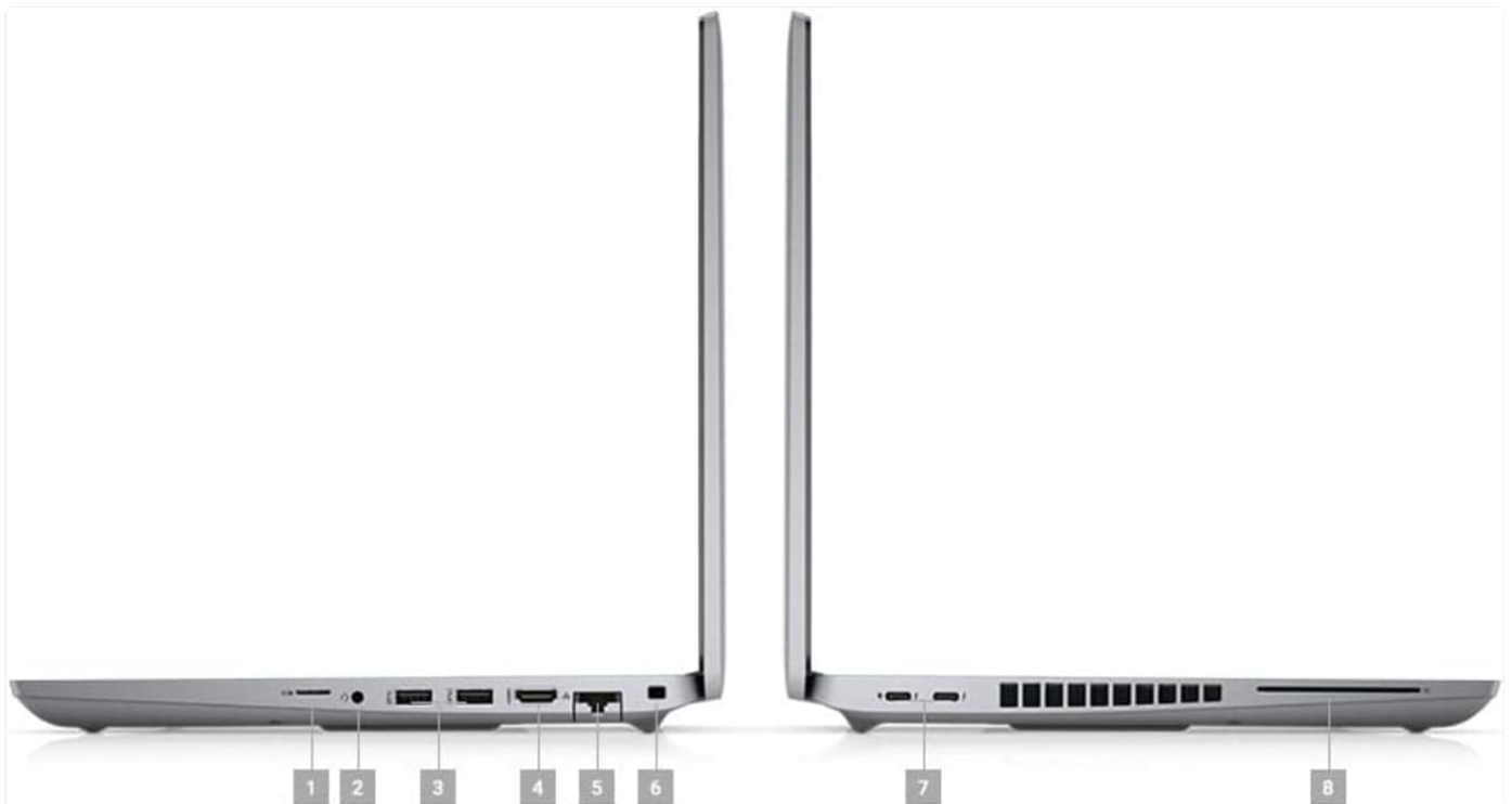
Figure 2: Left and Right Side Ports. This image details the connectivity options on both sides of the laptop, including USB, HDMI, Ethernet, and Thunderbolt ports.
