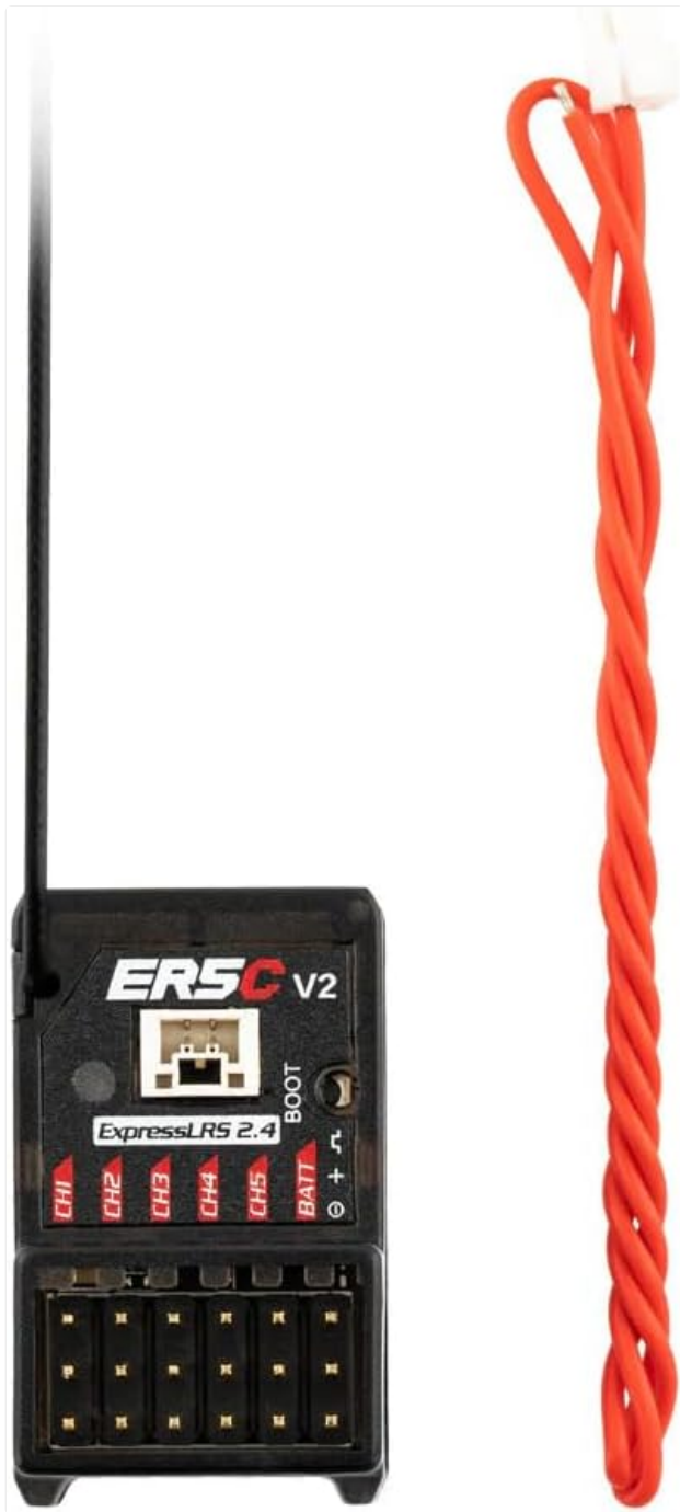
Figure 6: ER5C-V2 receiver with voltage telemetry wire. This image shows the receiver next to the dedicated wire used for external battery voltage telemetry, allowing monitoring of battery levels.
