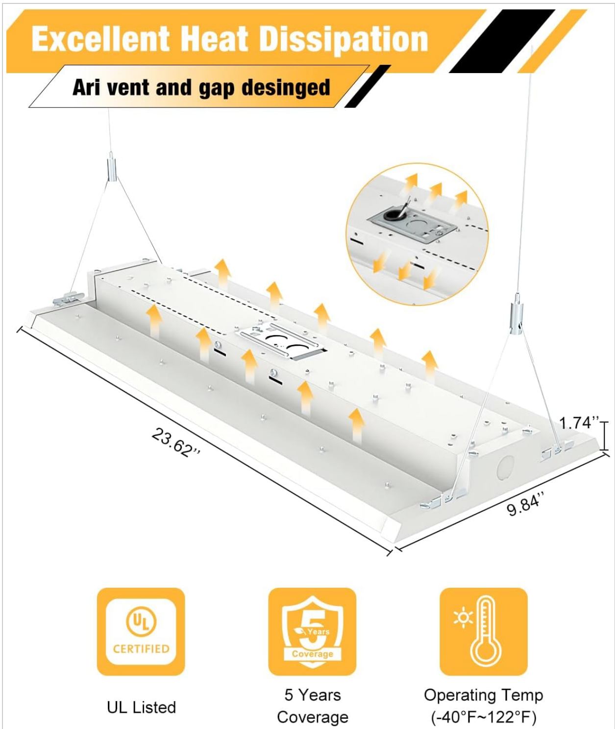
Image 4.1: Product dimensions and heat dissipation features.
