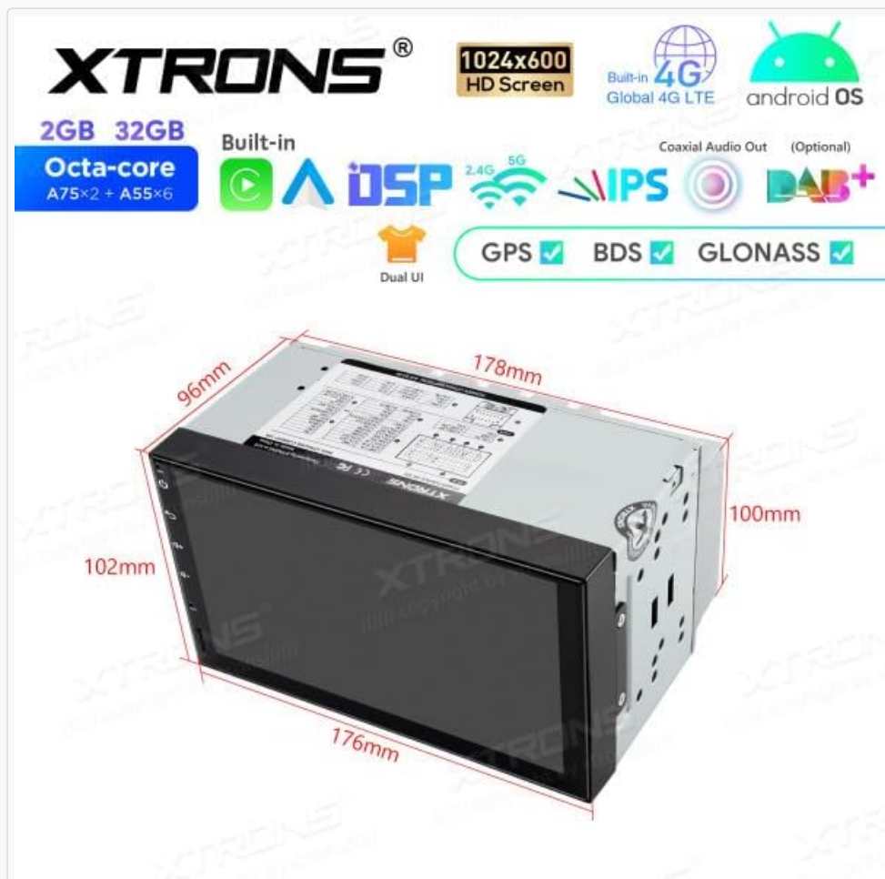
Image: Diagram showing the physical dimensions of the XTRONS TIE723L unit. The main body measures approximately 178mm in width and 100mm in height, with a depth of 96mm. The front panel measures approximately 176mm in width and 102mm in height.
