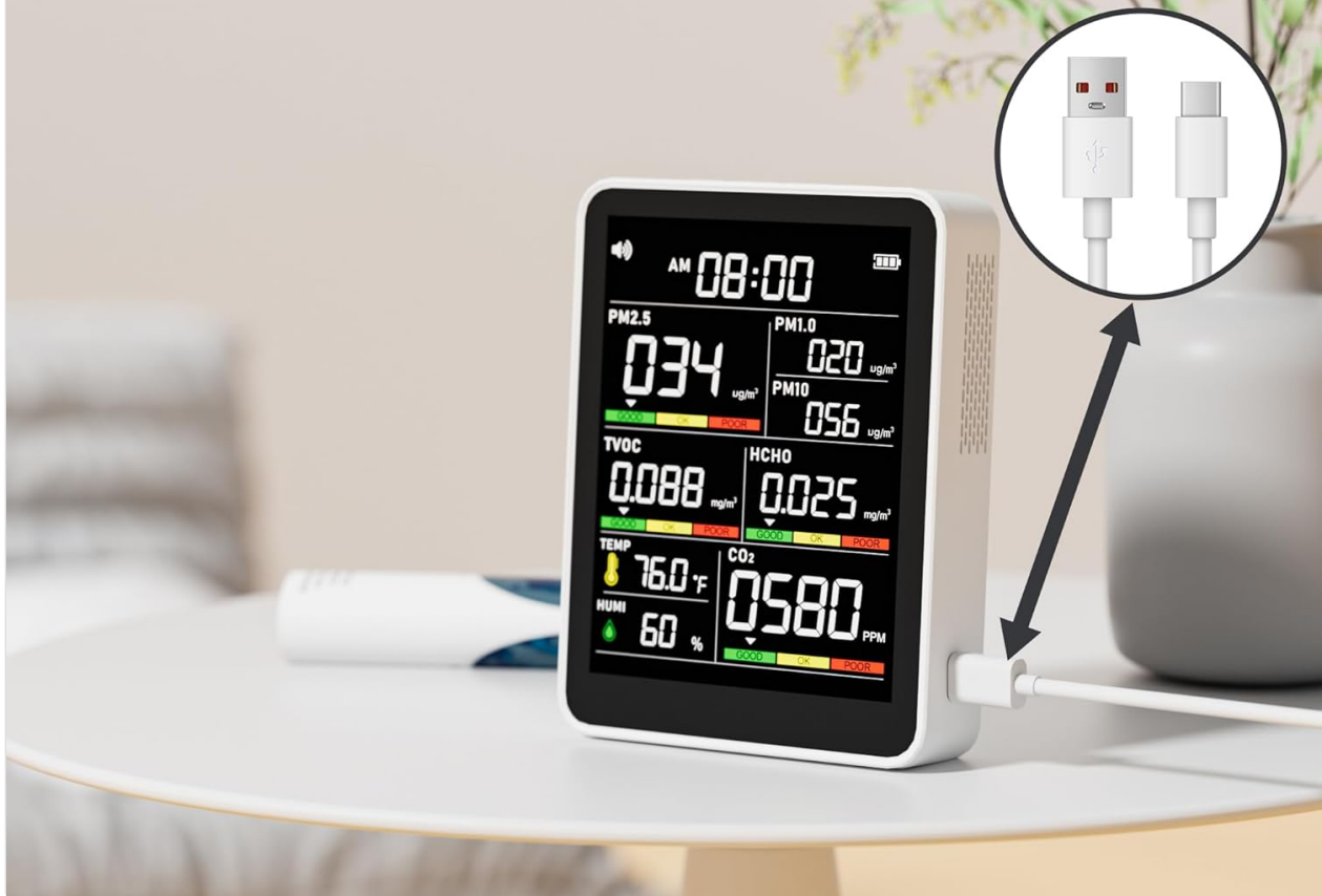
Image 4.1: The AIROASIS AK16 monitor being charged via its Type-C USB port, illustrating the connection point.
