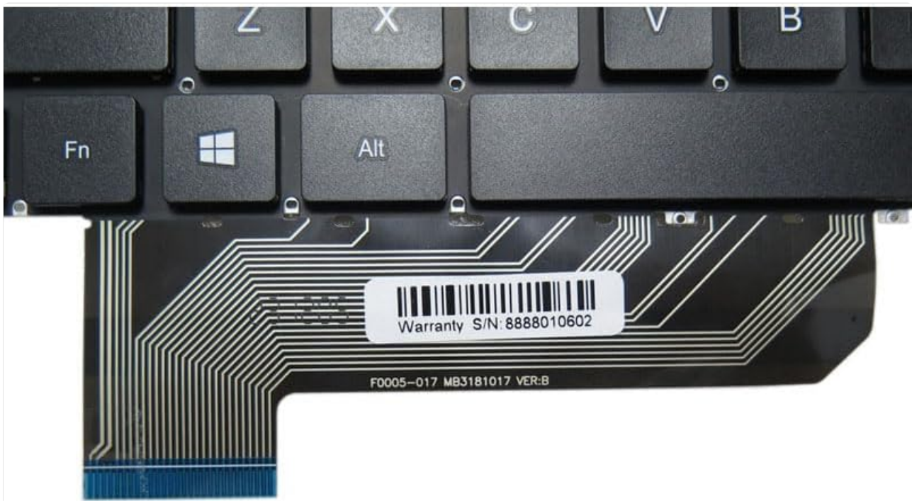
Figure 2: Detail of the keyboard ribbon cable with serial number.
